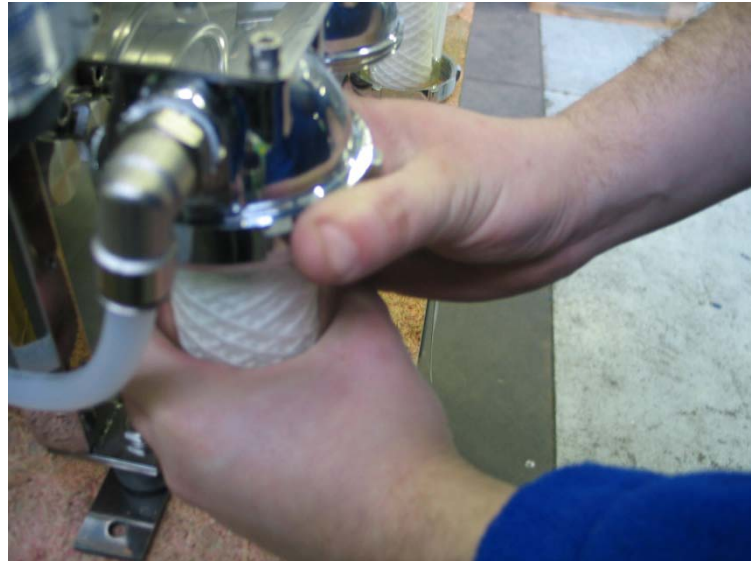
HAND POSITION FOR CHANGE THE FILTER
