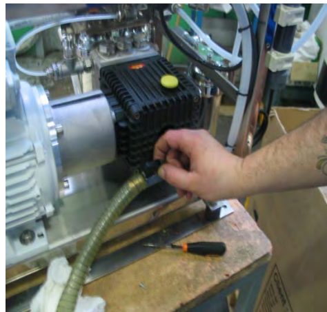
Open valve in position discharge for the connection on the hose for empty the pump
