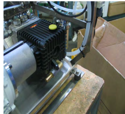
Valve closed and now underscrew the yellow cap for put on the pump the new oil
