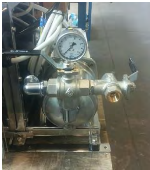
Turn the valve on fresh water position
