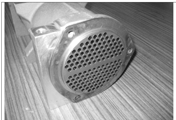
Fig. 108: Fitting the spacer sheet (example)
