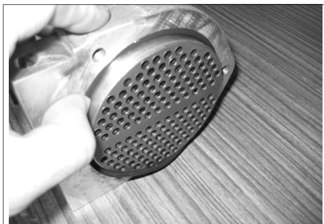
Fig. 107: Fitting the O-ring on the side opposite the water side (example)
