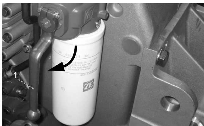
Fig. 77: Change lever in the 6 o'clock position (example)
