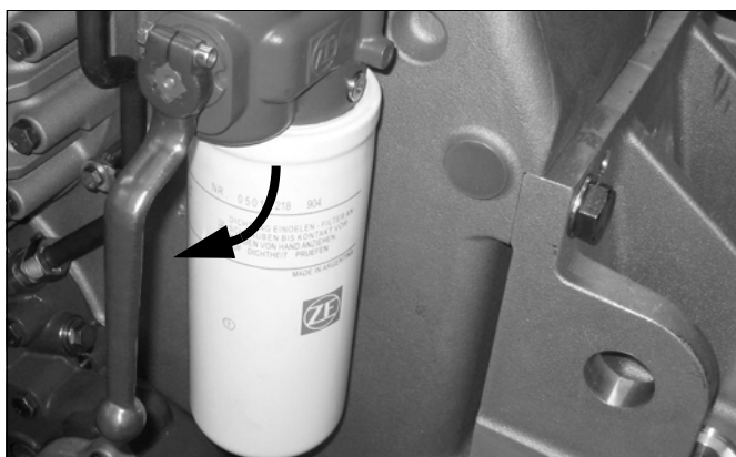
Fig. 54: Change lever in the 6 o'clock position (example)
