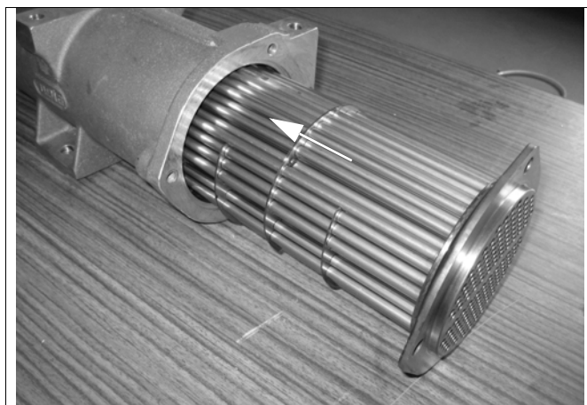
Fig. 106: Fitting the pipe bundle (example)
