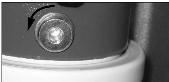
Fig. 52: Vent screw on the oil filter (example)
