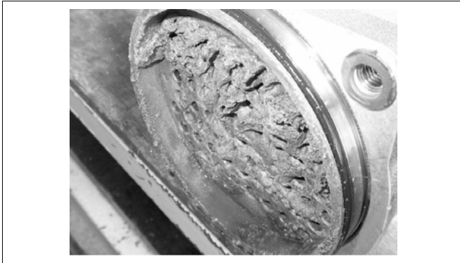
Fig. 31: Fouling: Organic deposits on the pipe bundle caused by a low flow velocity and a long standstill time (example)
