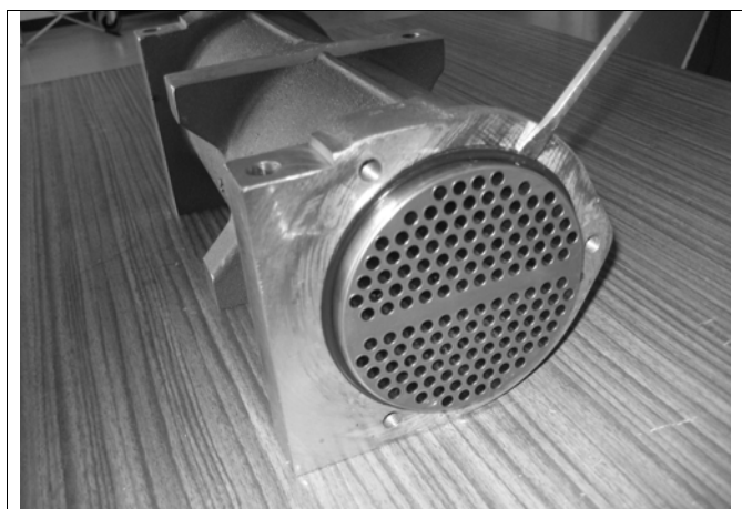
Fig. 101: Removing the O-ring on the side opposite the water side (example)
