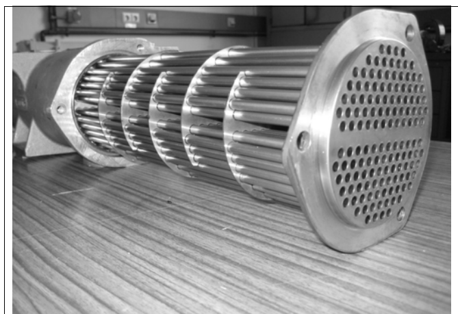
Fig. 102: Removing the pipe bundle (example)
