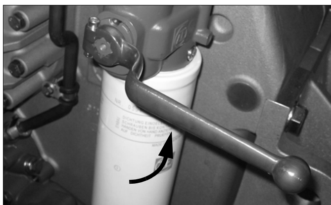
Fig. 51: Change lever in the 3 o'clock position (example)
