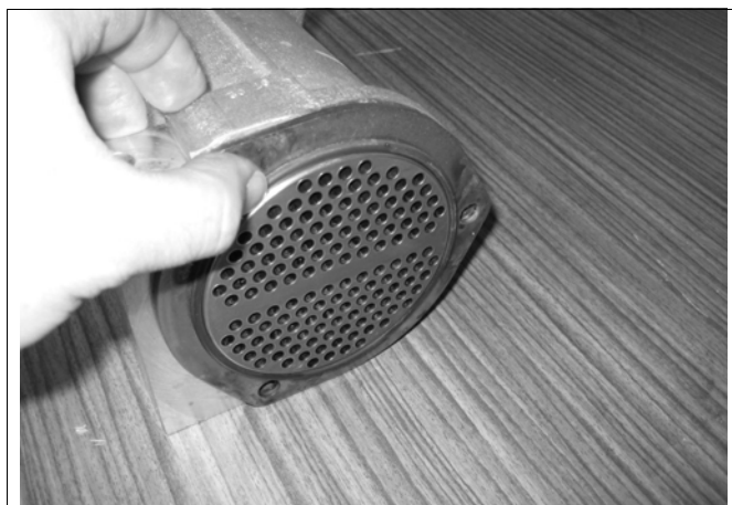
Fig. 104: Fitting the outer O-ring (example)
