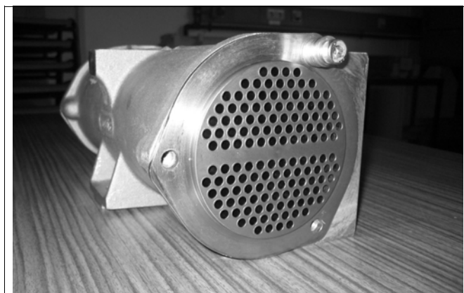
Fig. 97: Pipe bundle secured with one screw (example)
