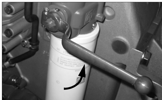
Fig. 76: Change lever in the 3 o'clock position (example)
