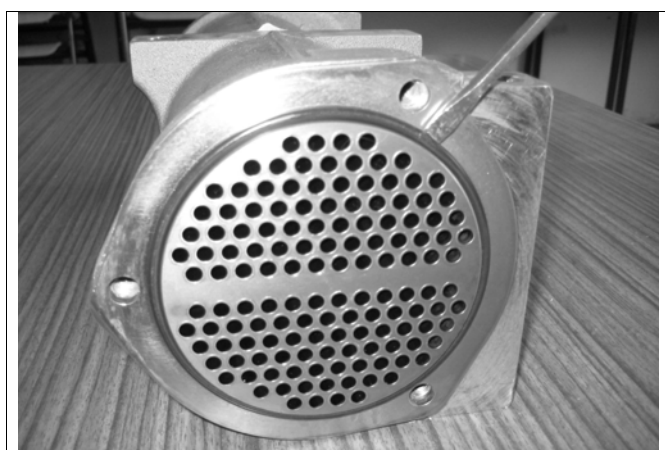
Fig. 99: Removing the O-rings (example)
