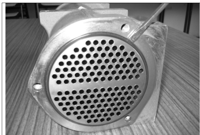
Fig. 96: Removing the O-rings (example)
