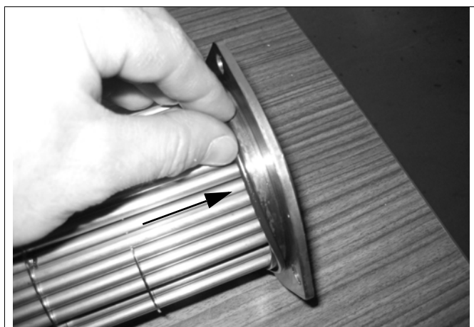
Fig. 105: Fitting the O-ring on the water side (example)
