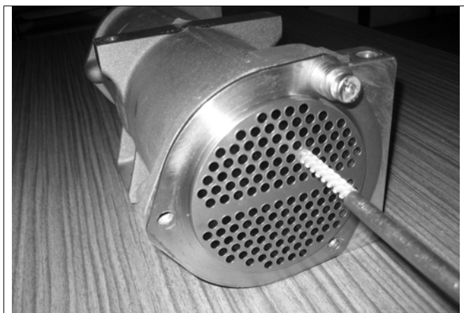
Fig. 98: Cleaning pipes with a nylon brush (example)
