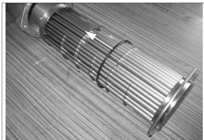
Fig. 103: Removing the O-ring on the water side (example)
