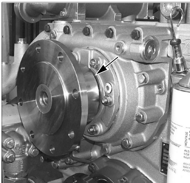
Fig. 111: Input shaft seal ZF 2150 V (example)
