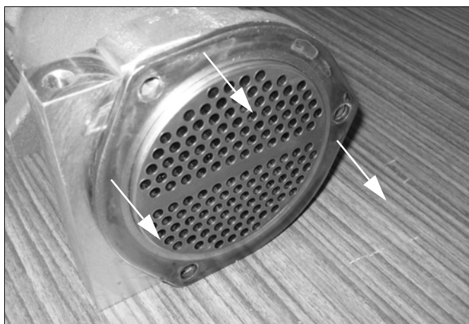
Fig. 100: Removing the spacer sheet (example)
