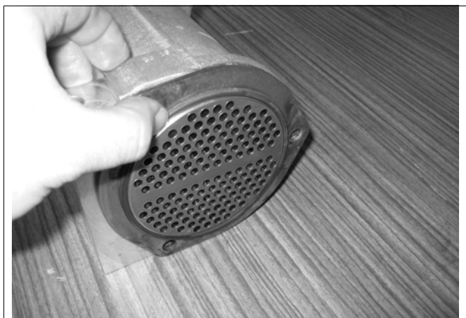
Fig. 109: Fitting the outer O-ring (example)
